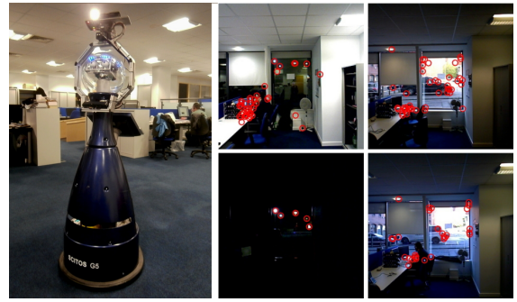
Fig. 4. The SCITOS-G5 robot patrolling the LCAS Witham Wharf office and example observations with extracted BRIEF features.
