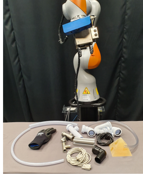
Fig. 1. The slave robot and an example of industrial objects from our dataset. The robot is an KUKA IIWA equipped with an eye-on-hand Ensenso RGB-D camera and a Schunk Parallel Gripper. The object are randomly selected from different categories: deformable, transparent, metallic, combined, and primitive 3D printed shapes.
