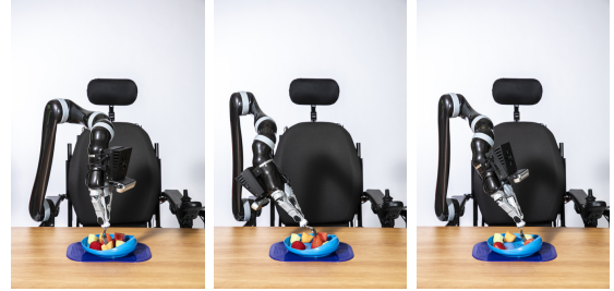
Fig. 1: A JACO robotic arm skewering food items in different configurations in a plate using a Vertical (left), Tilted-Vertical (middle), and a Tilted-Angled (right) skewering acquisition actions.
