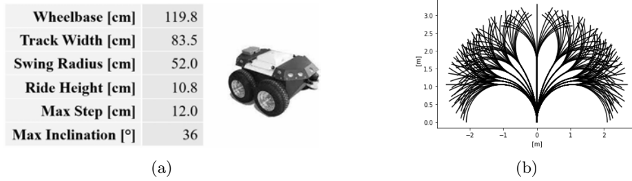
Fig. 3: (a) Seekur Jr. Robot (Courtesy of Generation Robots), and (b) portion of the robot action space for no initial point turn rotation.
