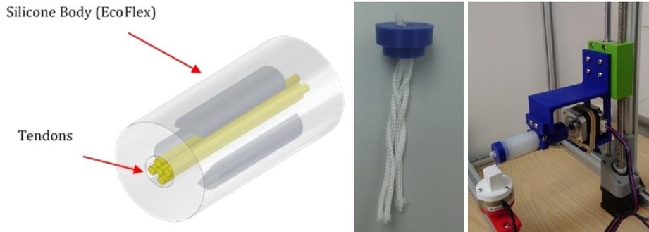
**Fig. 1.** Actuator construction from left to right: (a) Actuator design showing internal core, (b) braided polypropylene rope with end cap, (c) stepper motor twisting the tendons in the core.
