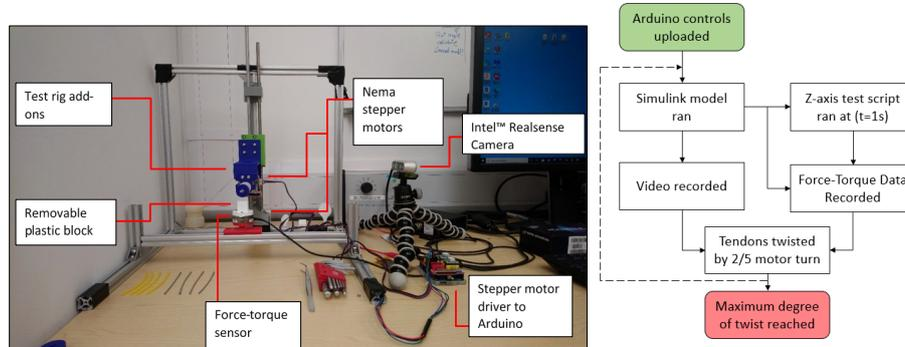
**Fig. 1.** From left to right: (a) components of the experimental setup, with the z-axis acting vertically, (b) simplified model of experiment procedure.
