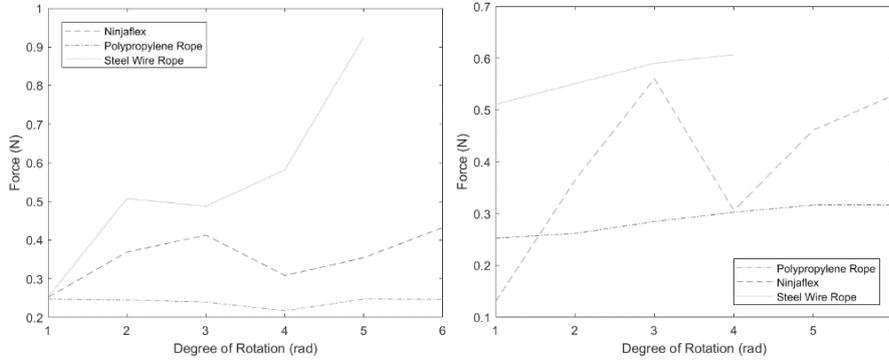
**Fig. 1.** Z-axis force-torque data plotted until second peak from left to right: (a) unbraided tendon configuration, (b) braided tendon configuration.
