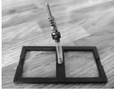
Fig. 3: Demonstrator consisting of a 3D-printed frame, an exchangeable steel spring and a variable amount of hex nuts for varying the mass.
