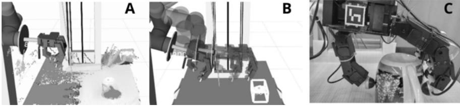
Fig. 1: Methodology for the calculation of force metric. **(A)** Point cloud data of the workspace. **(B)** Path planning towards the bounding box of the object. **(C)** Robotic hand position during metric calculation.
