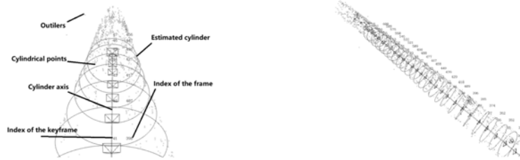
Fig. 4. The 3D points from actual data and the cylinder fit to them. The non-cylindrical points can be seen which are not fit to the cylinder, and the cylindrical points which will be fit to the estimated cylinder are seen ahead of the most recent keyframe.
