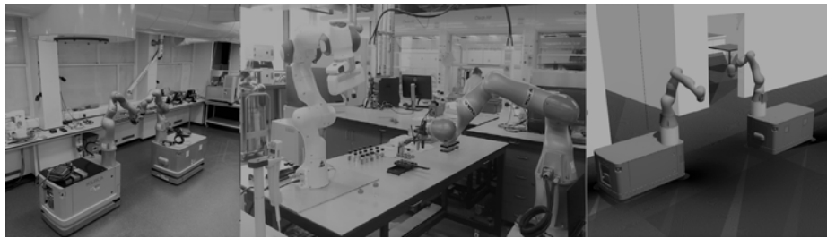
Fig. 4. (Left): Two KMR iiwa robots interacting with each other. (Centre): KMR iiwa placing the rack of vials in order for the Frank Emika robot to dispense liquid. (Right): two KMR iiwa robots interacting in Gazebo simulation environment.
